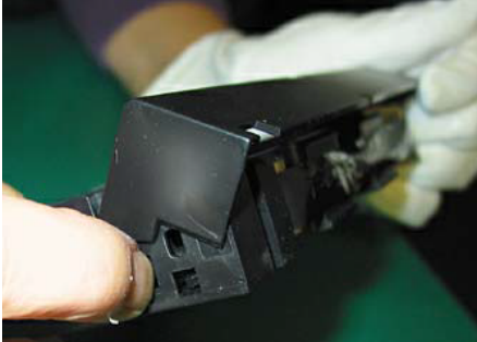
press and pull back anti-static guard - VHS
