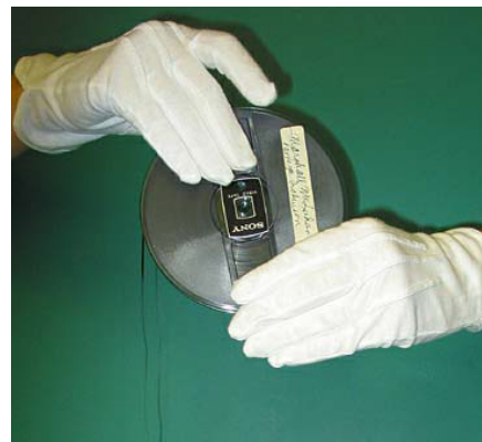
wind open reels by carefully turning reel
