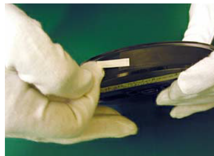
secure end with acid-free tape
