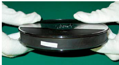
tape down ends of open reels
